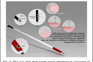
Fig. 1. The eye stick that sends sonic vibrations in response of visual structure & colour detected [4].
